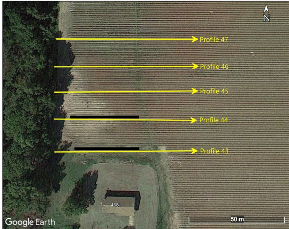
Figure 3. Google Earth satellite image acquired June 2016 showing a very large sand blow (light-colored soils) at site DBNW5, locations of GPR profiles 43, 44, 45, 46, and 47 (yellow lines), and locations of two paleoseismic trenches (heavy black lines).
